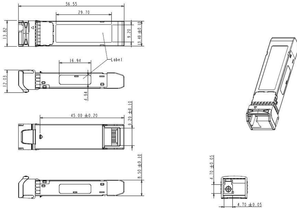
**Figure 3. Mechanical Specifications**
